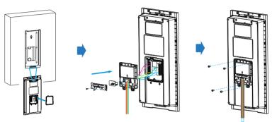
For convenient wiring, hang R28X on the wall-mounting box/ flush-mounting bracket with rope. Then insert the silicon rubber sealing ring into the groove.
