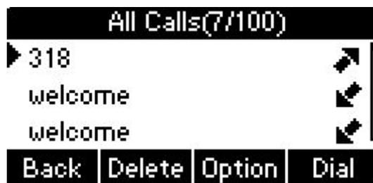
3. Press the Up or Down key on the phone keyboard to select the log.
