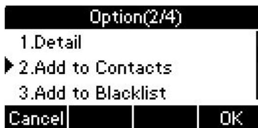
4. Select Add to Contacts, then press OK soft key to enter edit interface. After finish edit, press Save soft key to save the modify.
