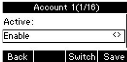
4. Press Down to enter the next item. Input the label, display name, register name, account, password and SIP separately.
