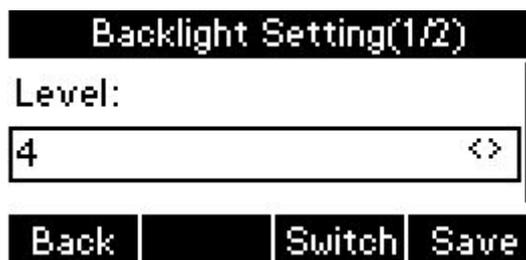
3. Press Down button to set the backlight time. Press Left or Right Key or Switch softkey to modify the backlight time. 30 seconds by default.
