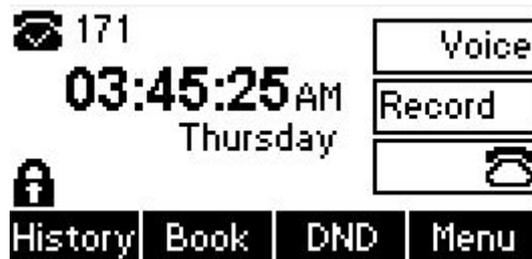
3) Anyone need to enter the password to unlock the keypad. If the password is incorrect, it will pop up a prompt box “Wrong PIN!”
