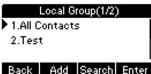
4. Input keywords such as name, any character of number or whole phone number, press the Search softkey or the OK key to enter the Search Contacts interface. For example, input "A", press Search soft key . It will show the name which contains A letter in the contact.
